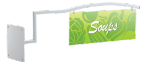
AM105 Curved 24" arm, 5-1/2" high step upright, 6" square mount.
